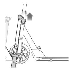
**2** Loosen the collar clamp and slide it upward.
