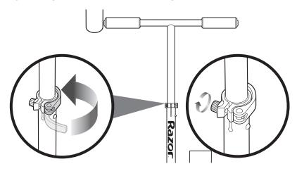
**1** The tension of the quick-release lever can be adjusted by manually tightening or loosening the Allen bolt. Be careful not to over-tighten. You should always be able to open and close the quick-release lever by hand and the T-bar should slide freely when the quick-release is open.
