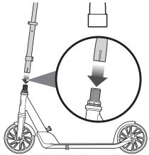
3 Insert T-bar into the fork until it bottoms out on the headset locknut.
