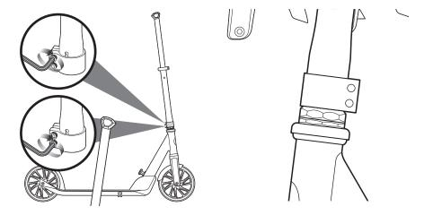
**4** With the front wheel pointed straight ahead and the handlebars square to the front wheel and the Razor logo facing the front, tighten the clamp as shown. Tighten securely.
