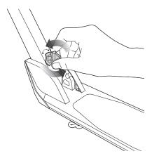
**1** To fold scooter you must first deactivate the antirattle feature. Twist the knob left until loose. No need to loosen knob more than one full turn.
