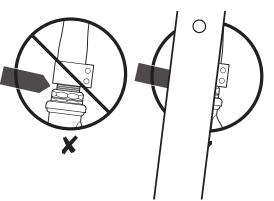
**WARNING:** Do not attempt to thread the handle bar into the front fork thread. Tighten clamp securely.
