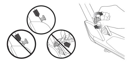
Note: To activate the anti-rattle feature twist the knob to the right to tighten. Please note there is no need to over tighten.
