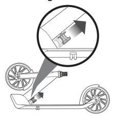
1 To release the folding mechanism, place the scooter on the ground, put one foot on the deck plate and pull the Anti-Rattle knob up. Raise T-bar up until it is securely locked in the upright position.
