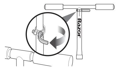
**2** To adjust the height of the handlebars, open the quick-release lever and slide the T-bar to the desired position and resecure the quick-release lever to lock into place.
