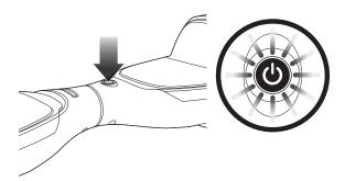
**2** Turn power **0N.** If product remains level or adjusts to become level, calibration has been confirmed. No further steps are needed.
