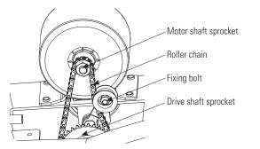
**Note:** Proper alignment of the chain must be maintained. If the chain is adjusted properly, but is noisy or rough running, check alignment of the sprockets. The drive-shaft sprocket can be adjusted slightly from side-to-side by loosening the set screw. Note that a key way maintains the drive position to the shaft.
