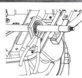
**8** Remove the two (2) "C" clips (one on each side). Remove the two (2) brackets that hold the rear axle in place and remove axle.
