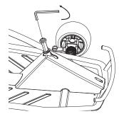
**1** Using a 5 mm Allen wrench, loosen the screw located in the steering column.
