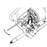
**3** Remove the eight (8) bolts (four on each side) that attach the brackets to the frame.
