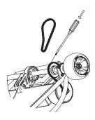
**3** Using a flat head screwdriver, carefully re-attach the clip on to the link plate. The clip must point in the drive direction of chain rotation.
