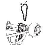
**2** Wrap the chain around both sprockets and tension idler. Insert the connector link all the way through the chain and fit the link plate over the connector link.
