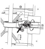
**2** If the adjuster is threaded outward and the brake still has too much slack, use the auxiliary adjuster at the rear brake for additional adjustments. Note: When properly adjusted, the brake lever will have approximately 3 mm of free play before the brake engages.
