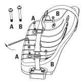
**1** Position the seat over the frame and align it with the holes in the frame. Align the safety belt anchor holes to the holes in the seat and frame with the lap/shoulder assembly on the left and the receiver latch on the right. Insert the four (4) seat bolts and tighten securely.
