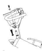
**2** Make sure the wires are not tangled. Insert the steering wheel, washer and screw into the steering column as shown.
