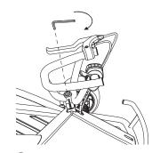
**3** Tighten screw securely using a 5 mm Allen wrench.
