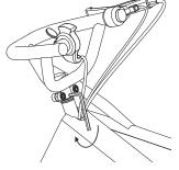
4 Using a 5 mm Allen wrench, alternately tighten each of the bolts on the steering wheel clamp. When the bolts are properly tightened, the gap between the clamp halves should be even.
