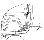
**2** Loosen the four (4) 5 mm bolts (two on each side) on the battery cover and remove cover.
