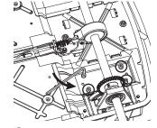
**6** Using a 5 mm Allen wrench, loosen the four (4) bolts holding the motor to the frame. Carefully lower the motor and remove chain from around the motor sprocket.
