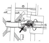
**5** Using a 10 mm wrench, loosen the nut that holds the brake cable and pull cable outward.
