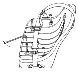
**1** Using a 5 mm Allen wrench, loosen the four (4) seat bolts and remove seat.
