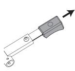
1 Using a Phillips screwdriver, loosen the screw on the spark cartridge and remove the cartridge.
