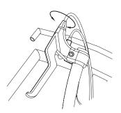
**1** To adjust the brake, thread the adjuster in or out 1/4 to 1/2 turns until the desired brake adjustment is attained
