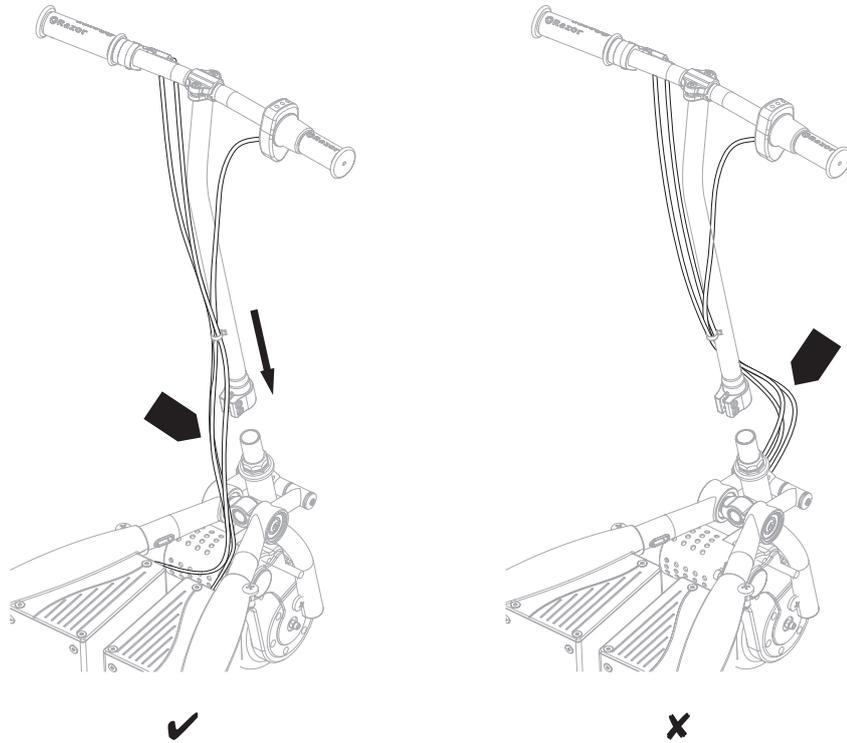
**1** Slide stem onto the front fork. Make sure throttle and brake cables are not touching the rotational corrector.
