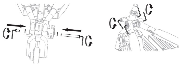
**5** Insert coupling bolt as shown and tighten using two (2) 5 mm Allen wrenches until secure.
