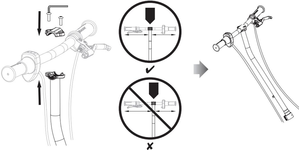
**1** Using a 5mm Allen wrench, remove the 2 bolts on the handlebar clamp.
