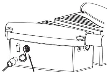
**2** Turn the power switch OFF before charging. Plug the charger into the charger port on the side of the battery compartment.
