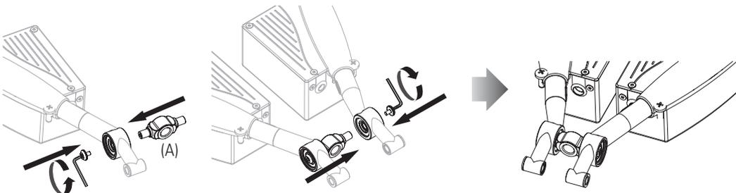
**1** Insert the rotational connector (A) into the right leg tube as shown. Using a 5mm Allen wrench, slightly tighten bolt to hold connector (A) in place.
