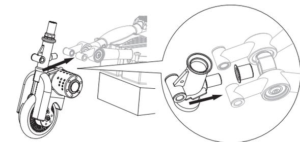
**4** Insert the front fork into the rotational connector.
