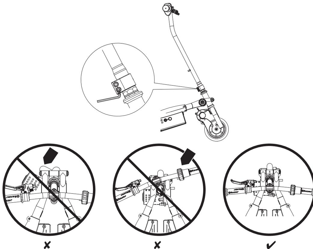
**2** Align the front wheel with handlebars using a 5mm Allen wrench. Tighten bolts on collar clamp until collar clamp is secure.
