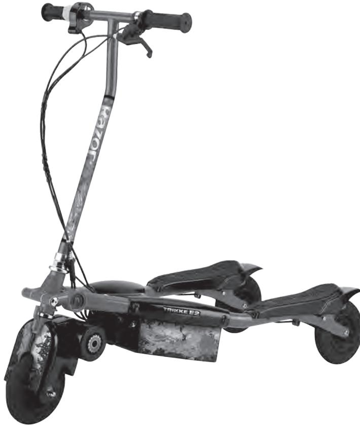
**⚠ NOTE:** The Trikke E2 must be traveling up to 3 mph before motor will engage. Kick start up to 3 mph while applying the throttle to engage motor.
