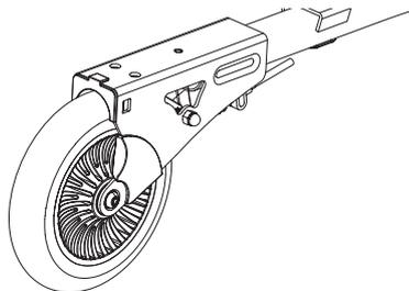
**1** Using two (2) 5mm Allen wrenches, loosen axle bolt and remove wheel. Install new wheel, re-insert axle bolt and tighten securely.
