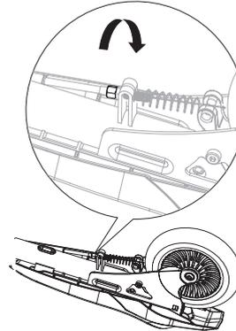
**1** To adjust the brake cable tension, thread the brake lever adjuster in or out 1/4 to 1/2 turn until the desired brake adjustment is attained. Most adjustments are complete at this step. If brake needs further adjustment, proceed to step 2.
