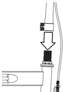
**1** Place the handlebar stem on the front fork.
