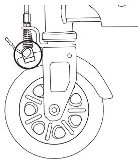
**3** If the brake is too tight or too loose, use a 8 mm wrench and a 3 mm Allen wrench to make adjustments as needed.
