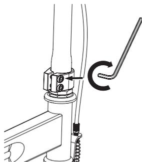
**2** Using a 5 mm Allen wrench to tighten the two (2) bolts on the collar clamp. The collar clamp is properly tightened when the handlebars cannot be twisted out of alignment with the front wheel. Make sure the handlebars are in line with the front wheel before tightening the bolts all the way.
