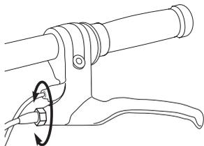
**1** To adjust the brake cable wire, thread the brake lever adjuster in or out 1/4 to 1/2 turn until the desired cable tension is attained.
