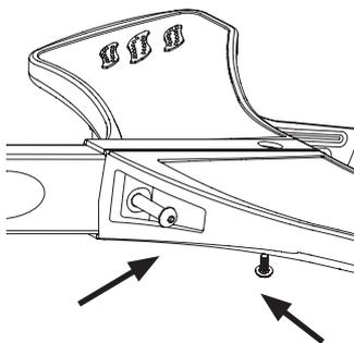
**4a** If necessary, use a mallet / hammer to tap the two coupling bolts until they are all the way through the platforms.
