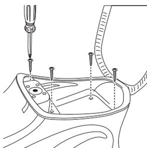
**1** Lift up the seat and unscrew the four (4) Phillips head screws in the storage compartment and remove the tray.
