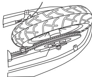
**5** Install the new chain or wheel by slipping the chain around the axle. Slide the axle into the slots on the frame. Slide the wheel forward and maneuver the chain onto the rear sprocket, motor shaft and chain tensioner.
