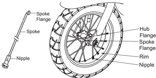
**1** Verify spoke tension by grasping and shaking each spoke. Spoke should not be loose from hub. Look for any play between spoke flanges where it mates with hub. Try to turn nipple using your fingers. You should not be able to spin any nipple by hand. If one or more spokes are loose, or if you can turn any nipple using your fingers, all spokes must be checked and need to be tightened with a spoke wrench.
