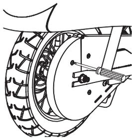
**8** Re-attach the chain guard. Test ride and readjust as needed.
