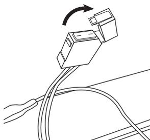
**2** Locate fuse box on top of battery. Open the fuse cover to expose the fuse.
