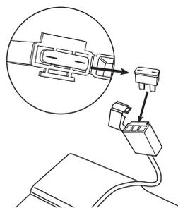
**3** Remove the fuse and replace with a new one of equal amperage.
