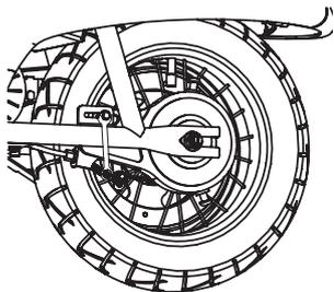
**7** Tighten the brake housing anchor securely.
