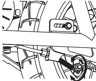
**1** To adjust the play, thread the brake lever adjuster on the hand brake in or out 1/4 to 1/2 turn until the desired brake adjustment is attained. Most adjustments are complete at this step. If brake still needs further adjustment, proceed to step 2.
