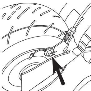
**10** To hook up the brake housing anchor, align the cable guide adjuster and install the spacer and bolt. Do not tighten until final step.
