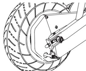
**2** Push open the access cover and align the access hole in the drive sprocket with the tire valve. Thread the adapter completely onto the valve and attach the pump and inflate to the PSI indicated on the tire sidewall. Push the access hole cover back.
