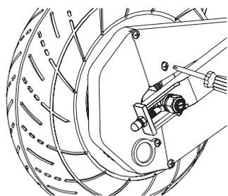
**1** Loosen screws and remove chain guard.
