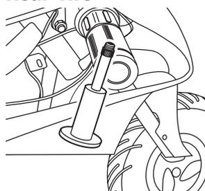
**1** Remove valve extender/adaptor from right handgrip.
