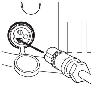
**1** Plug the charger port into the port on the electric motor bike. The charger works with the power switch in either the on or off position.
