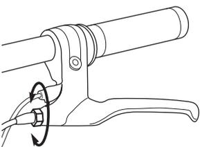
**1** To adjust the play, thread the brake lever adjuster in or out 1/4 to 1/2 turn until the desired brake adjustment is attained. Most adjustments are complete at this step. If brake still needs further adjustment, proceed to step 2.
