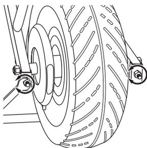
**9** Start screwing on both nuts alternating 1/8 to 1/4 turn at a time until chain is properly tensioned.
