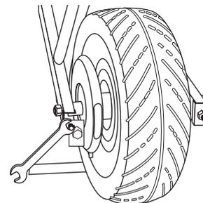
**4** Loosen and remove both axle adjuster nuts.
