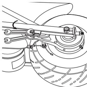
**3** With two 8mm wrenches, loosen brake housing anchor and disconnect. Keep the spacer and washers together.
