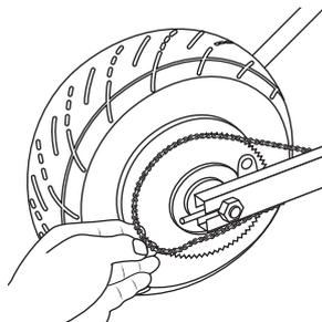
**7** Install the new chain or wheel by slipping the chain around the axle. Slide the axle into the slots on the frame. Maneuver the chain onto the rear sprocket and front sprocket.
