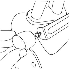
**1** Remove two rubber protectors from fairing mount. Remove two button head screws with rubber washers from both sides of fairing mount.
