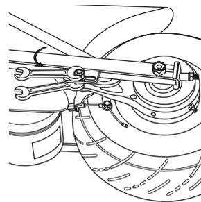
**12** Tighten the brake housing anchor securely. Re-attach the chain guard. Test ride and check. Readjust as needed.
