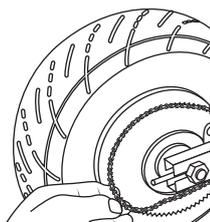
**6** Pull the wheel out. Note the arrangement of the hardware sequence.
