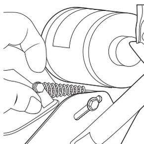
**11** Install the brake spring and thread the cable wire into the cable anchor. Thread the cable to its original position and tighten securely.
