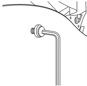
**2** Position the fairing and align holes with holes in fairing mount. Attach fairing to mounting points and secure with screws.
