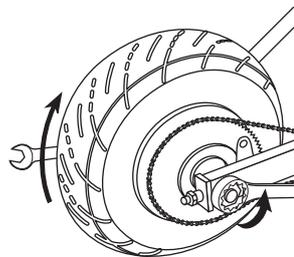
**5** With two 17mm wrenches, loosen the axle. Push the wheel forward to loosen the chain and remove from rear and front sprocket.
