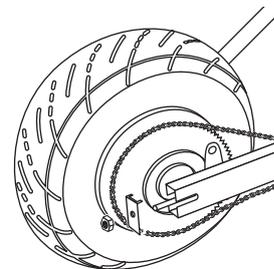
**8** Slide rear frame cap on axle adjuster bolt.
